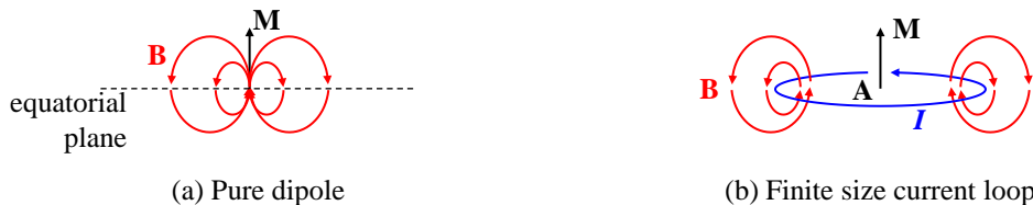
Figure 6.3 (a) Pure dipole B-field points down everywhere in equatorial plane. (b) Finite-size current loop B-field points up inside loop.
