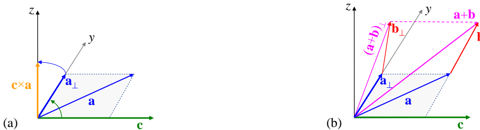
Figure 18.3 (a) Construction of a cross product. (b) The cross product of a sum: The projection of \mathbf{b} slides its tip to the y - z plane.
